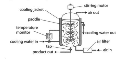
(i) Explain the function of the temperature monitor and cooling jacket.
